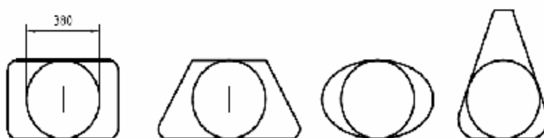
Figure 1 — Measurement of minimum clear opening
